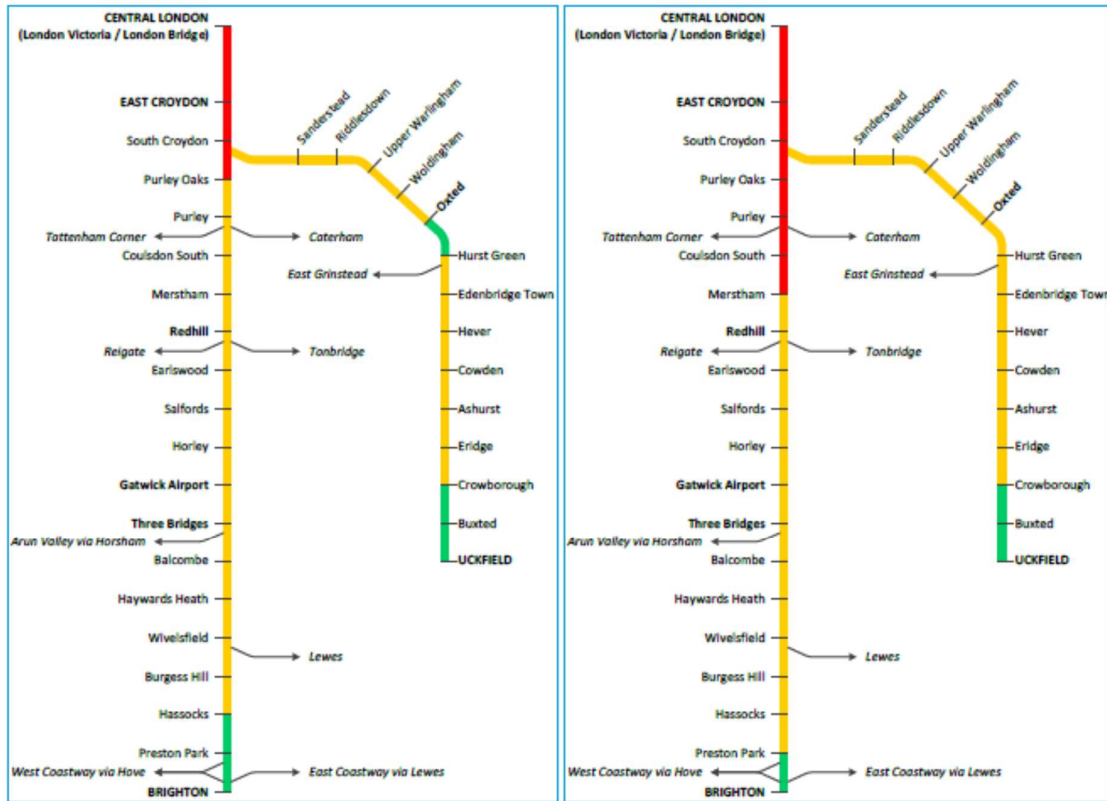
Figure ? “Do nothing” scenario without Housing development on the left and with Housing development on the right [morning peak period, 2043]; Red line: demand is in excess of capacity including standing spaces; Amber: demand is greater than seating capacity with standing required.
